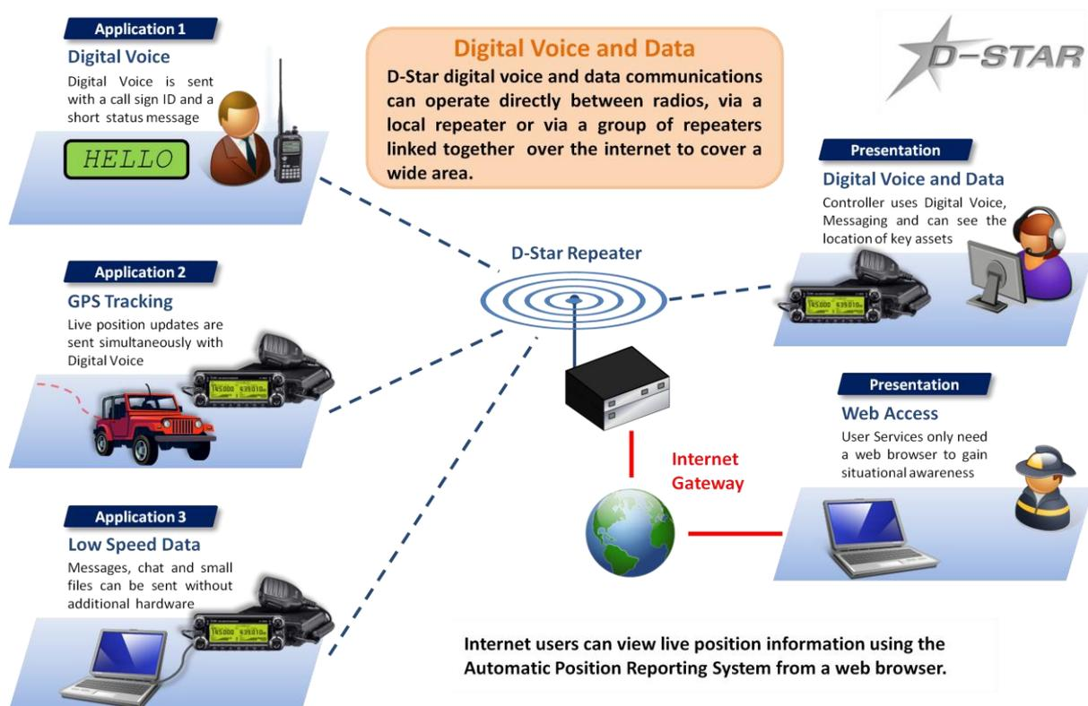
Two types of GPS data are supported: GPS mode is intended to provide a display the distance and bearing of the received station; whilst GPS-A mode sends the data in a more compact format intended for APRS tracking – although both formats are converted by the repeater software and posted as position reports on the APRS Internet Service, the latter is more reliable.
